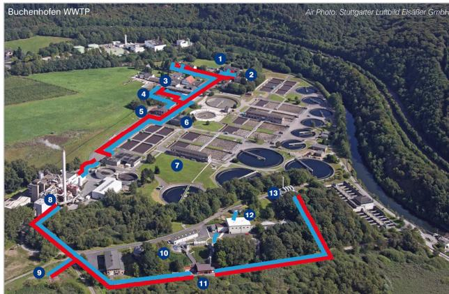
Figure 1. Local heat grid at Buchenhofen WWTP
